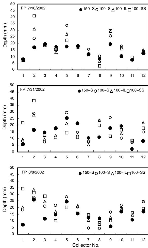
Figure 5. Individual collector measured depths under the fixed plate (FP) sprinkler package from the 16 July, 31 July, and 8 August 2002 test events for the 150-S collectors, and the 100-S, 100-IL, and 100-SS IrriGage arrangements.
