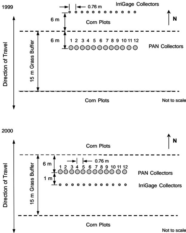
Figure 2. Field set up of the IrriGage and PAN collectors in 1999 (top) and 2000 (bottom).
