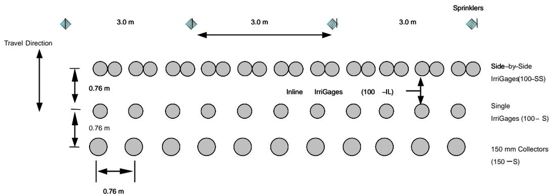
Figure 3. Field setup of the 150-S collectors, and the 100-S, 100-IL, and 100-SS IrriGage arrangements used in the 2002 tests.
