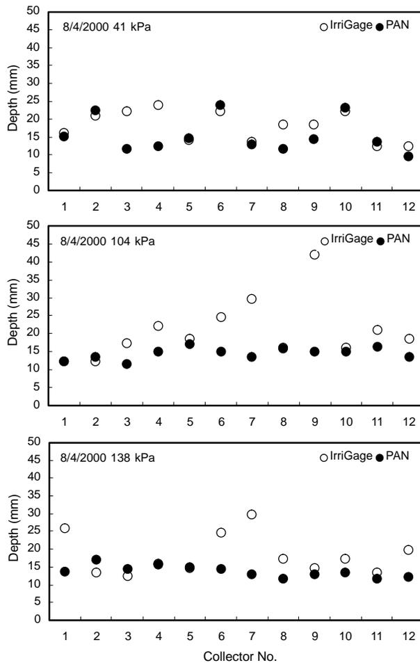
**Figure 4. Individual collector measured depths from the 4 August 2000 test event for both IrriGage and PAN collectors under the 41-, 104-, and 138-kPa sprinkler packages.**
