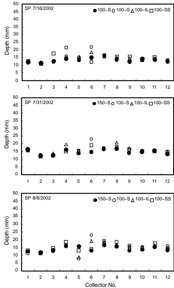
Figure 6. Individual collector measured depths under the spinning plate (SP) sprinkler package from the 16 July, 31 July, and 8 August 2002 test events for the 150-S collectors, and the 100-S, 100-IL, and 100-SS IrriGage arrangements.
