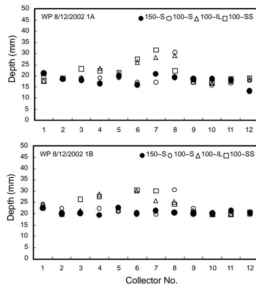
Figure 7. Individual collector measured depths under span 1 of the wobbling plate (WP) sprinkler package from the 12 August 2002 test events (1A and 1B) for the 150-S collectors, and the 100-S, 100-IL, and 100-SS IrriGage arrangements.
