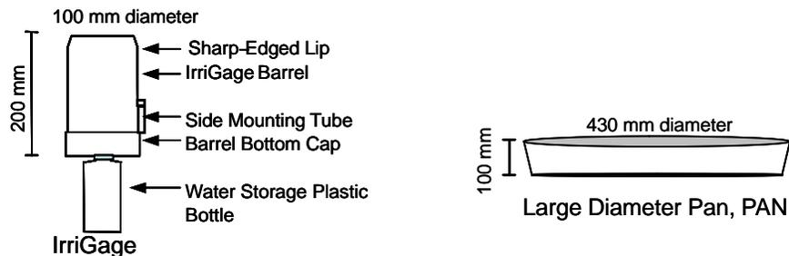
Figure 1. Characteristics of the 100-mm IrriGage and PAN collectors.
