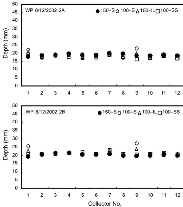
**Figure 8. Individual collector measured depths under span 2 of the wobbling plate (WP) sprinkler package from the 12 August 2002 test events (2A and 2B) for the 150-S collectors, and the 100-S, 100-IL, and 100-SS IrriGage arrangements.**
